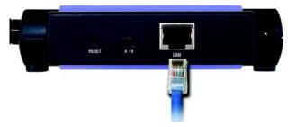
Figure 4-1: Connect the Ethernet Network Cable
